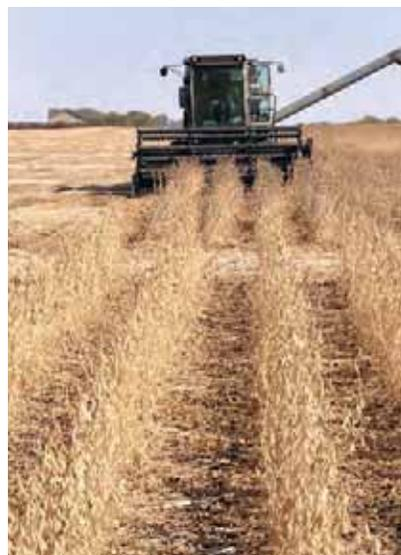
A Gleaner K2 combine, equipped with electronic weight and moisture gathering equipment, harvests a soybean plot at the Wabasso, Minn. site.
